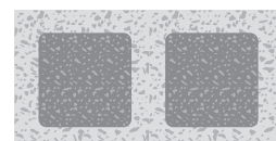
400 x 200 x 200mm block Block Compressing Strength: 12MPa Grout Compressing Strength: 20MPa
